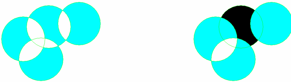
Fig. 4. Sensing coverage overlapping and non-overlapping regions a) before and (b) after node failure.
