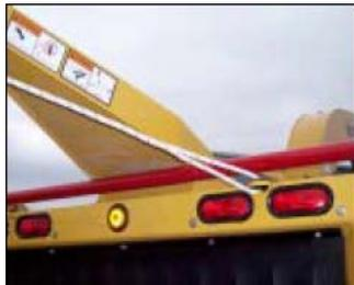
Winch line Safety Interlock and Storage Hook
