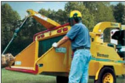
The investigation revealed that the location of the winch boom directly above and in front of the feed rollers, coupled with the simultaneous operation of the feed rollers, created this fatal "struck-by" hazard.
