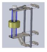
A prototype of the wave energy converter has demonstrated effectiveness in converting up-and-down wave motion to rotation.
