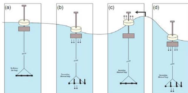
Conceptual operation of the tethered ballast point absorber system, shown as a wave moves right to left.
