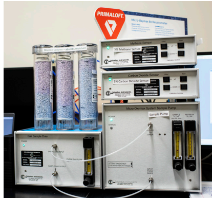
A Micro-OxyMax respirometer used to measure concentration of carbon dioxide and methane produced during biodegradation process
